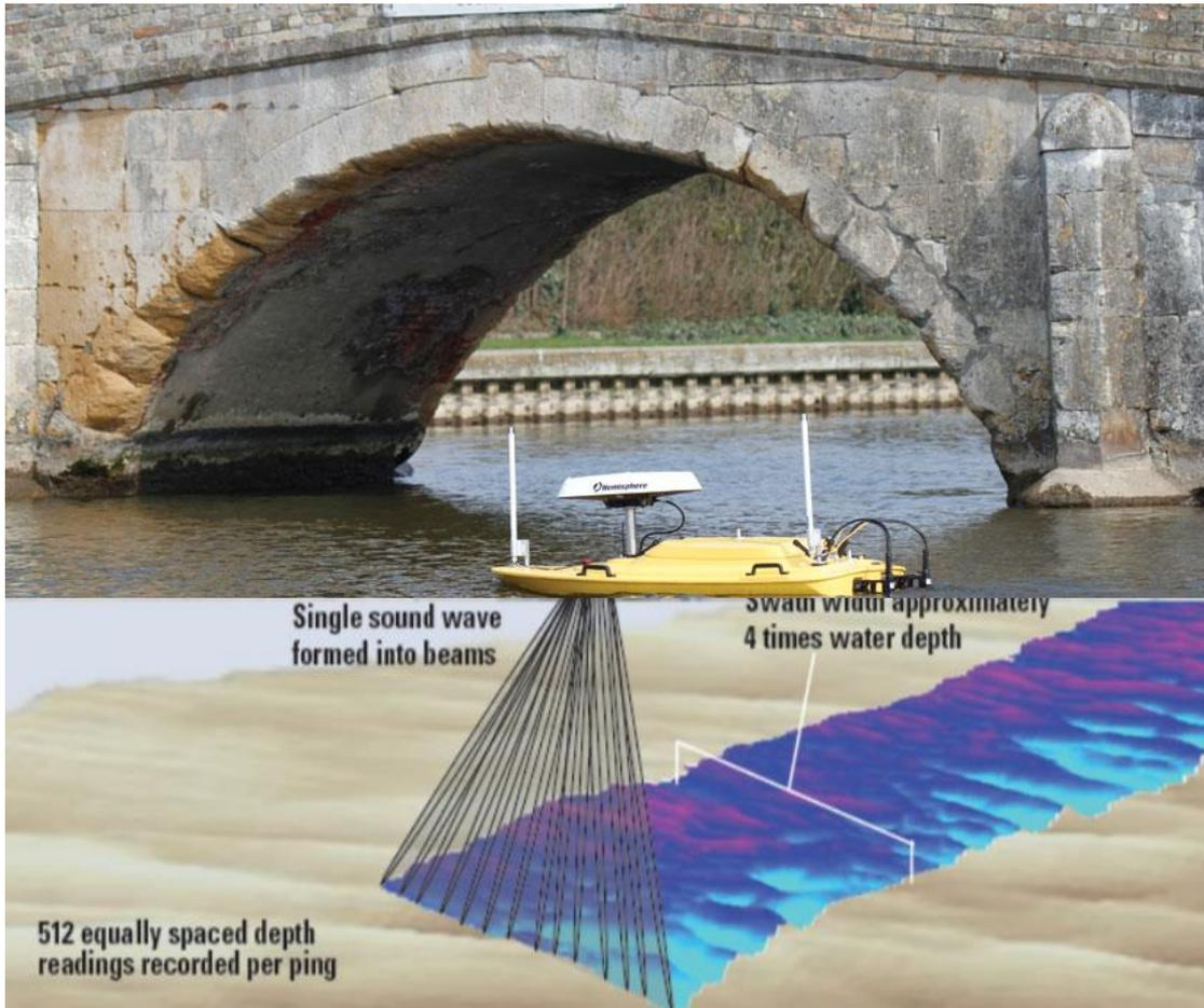
The Multi-Beam Echo Sounder beam width is typically four times the water depth. So a river of 8m depth could be surveyed with a swath footprint of 40m.
